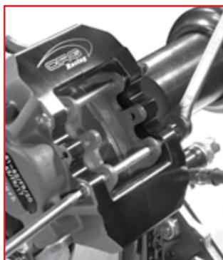
2. Using a 4mm allen key and a 8mm spanner loosen the fixing bolts.
