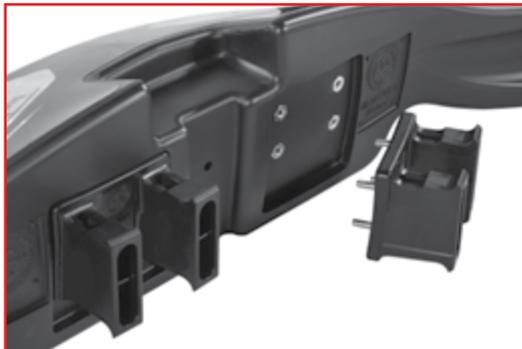
1. Attach the first fixing plate to the plastic spoiler using the four M6 bolts.
