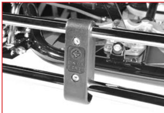
4. Using the two M6 bolts attach the two plastic halves of the clamp together.
