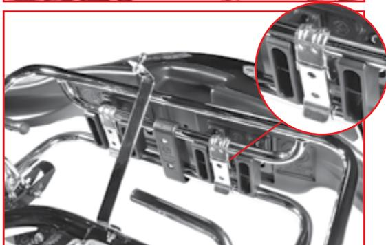
5. Close the bumper clamps and make sure the complete spoiler doesn't move.
