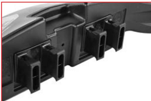
2. Attach the second fixing plate to the plastic spoiler using the remaining four M6 bolts.
