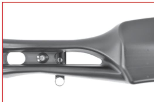
3. Attach the plastic rear bumper to the supports on the chassis using the M8 countersunk bolts and washers supplied.
