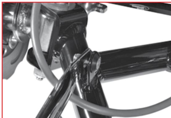
3. Attach the top front bumper using the M6 countersunk bolts and washers on the two points.
