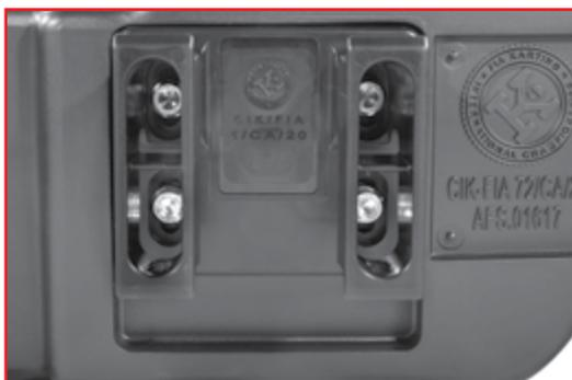
3. Make sure the fixing plate is fixed in the middle position.
