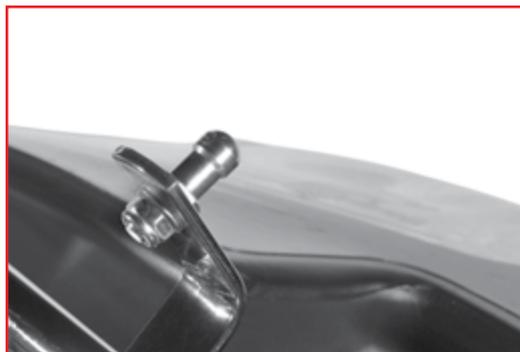
3. Attach the three front fairing pivot supports to the brackets.
