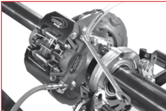
3. To bleed the brake: The pedal should be pushed down gently so the oil can pass through the system. When the pedal is down you should open the bleed valve on the caliper as shown in the picture and the air will come out of the tube attached to the bleed valve.
