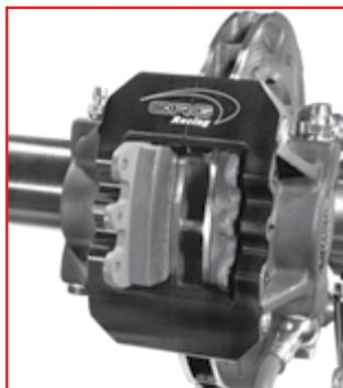
4. Pull out the brake pads and exchange with the new ones and then put the fixing bolts and safety clip back on the caliper.
