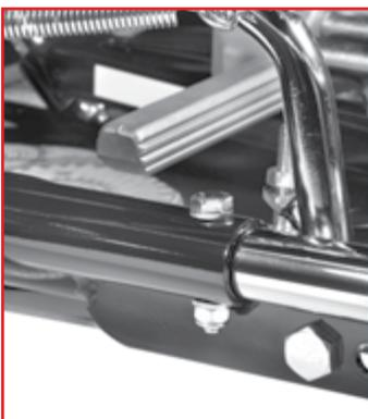
2. Tighten the bolt so it doesn't turn.
