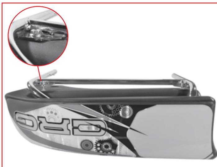
2. Fix it in place with the supplied screws.
